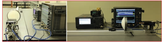
▲ Fig. 5 OTA quasioptic transmission at 285 GHz with 30 GHz bandwidth, receive side.
