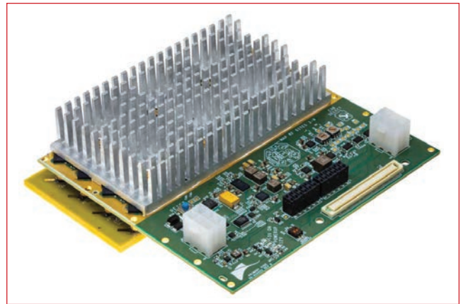
▲ Fig. 7 A planar phased array front-end with component side heat sink.
