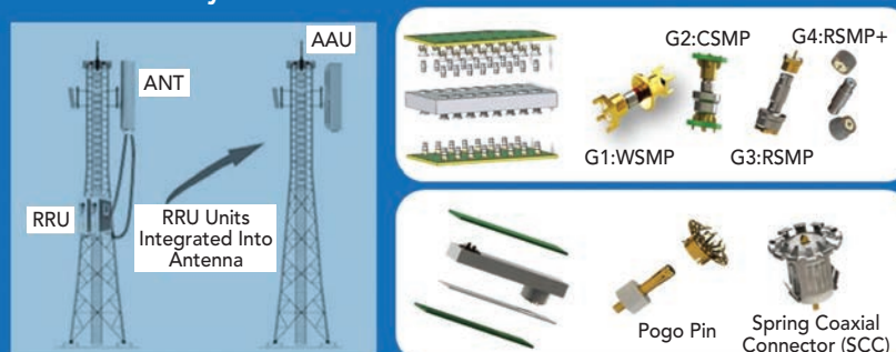
▲ Fig. 9 Suzhou Recodeal RF SMP BTB solutions for 5G (Source: Suzhou Recodeal Interconnection System Co., Ltd.).
