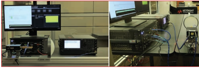
▲ Fig. 3 OTA quasioptic transmission at 285 GHz with 30 GHz bandwidth, transmit side.
