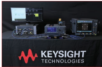
▲ Fig. 1 Sub-THz test bed for 220 to 330 GHz. measurements with waveguide connected to waveguide.
