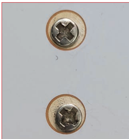
▲ Fig. 1 Potential tolerance issues arising from screw or pin alignment with machined holes in a PCB.
